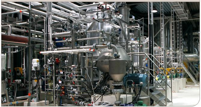
Increased yield, higher product quality and a more sustainable process were some of the improvments Swedish pulp producer Södra Cell experienced when upgrading the tall oil plant in its Värö mill to a TOPP5000 system. The new plant was supplied by HEAD Engineering and is based on Alfa Laval high-speed separators.
